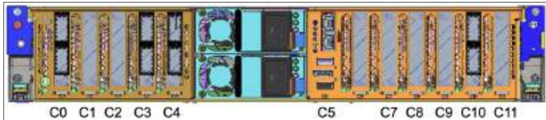
Figure 3-2 PCIe adapter slot locations on the Power S1122 and Power L1122 server models
