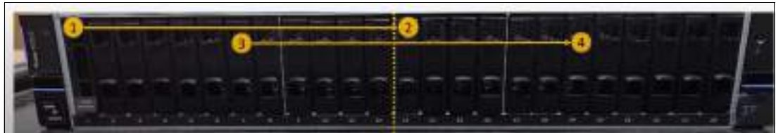
Figure 3-18 Drive installation order
