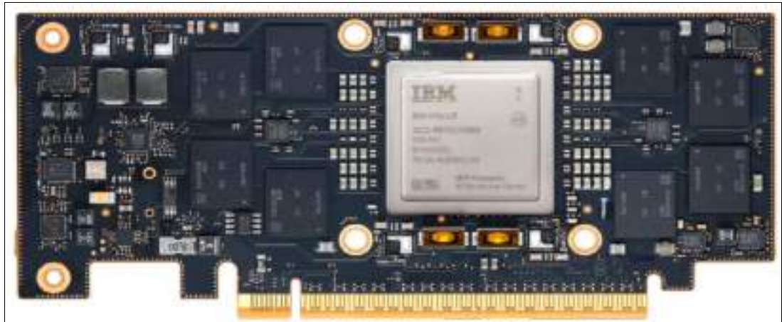
Figure 1-13 IBM Spyre Accelerator
